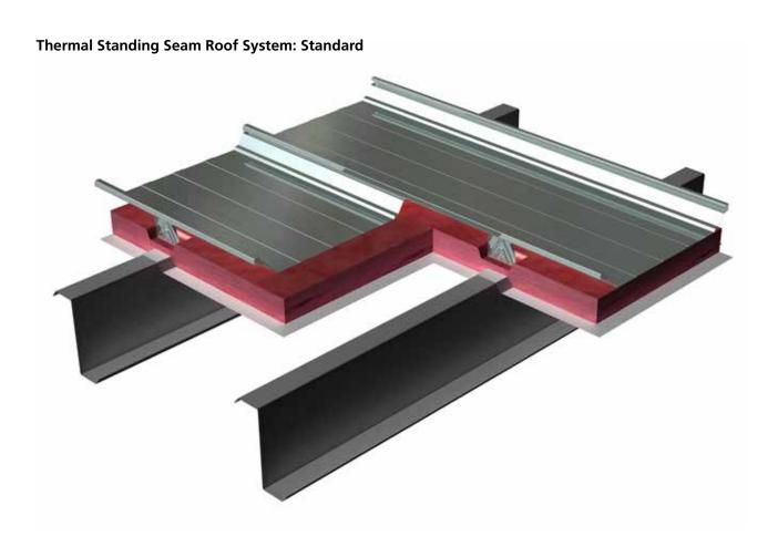
Purlins at 5'-0", RTL-24 roof, faced insulation draped over purlins
