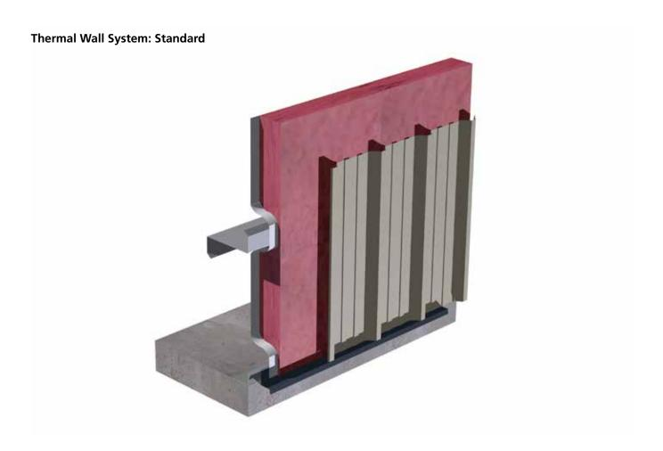
Girts at 5'-0" minimum, StormSeal panel with faced insulation draped outside wall girts
