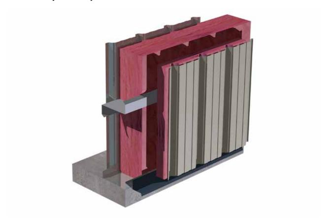
Girts at 5'-0" (minimum spacing), StormSeal exterior panels (wide rib out) with interior liner
