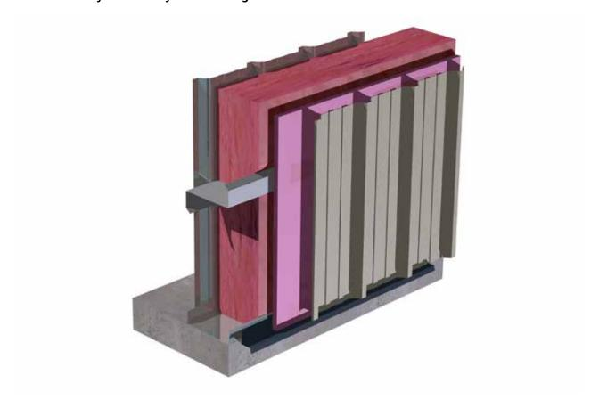
Girts at 5'-0" (minimum spacing), StormSeal exterior panels with interior liner
