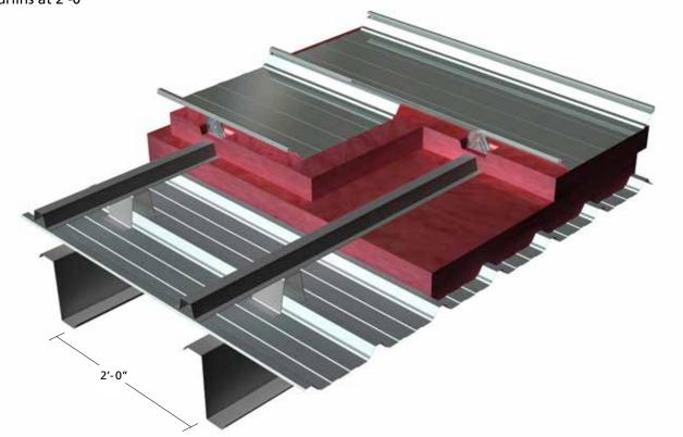
Purlins at 2'-0" with chairs spacing of 48" o/c, RTL-24 roof
