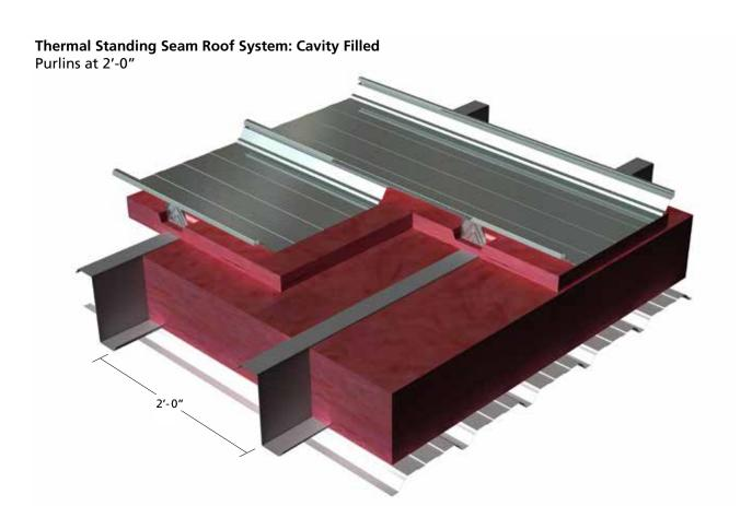
Purlins at 2'-0", RTL-24 roof with liner
