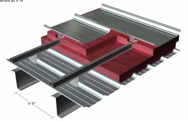
Purlins at 5'-0" with chairs spacing of 48" o/c, RTL-24 roof
