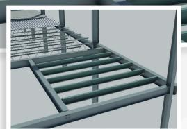
Above: Composite deck on open web steel joist are used in this large span mezzanine.
